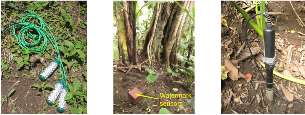
Figure 3.3: Images of (a) watermark sensors, (b) tree at forest site, (c) profile probe with access tubing
